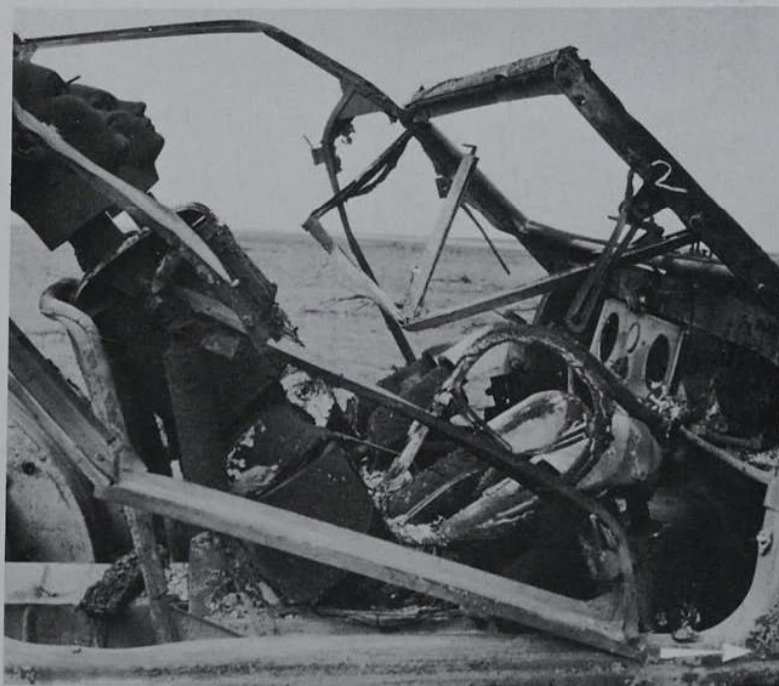
FIGURE 17. ROUND 3 . CHAMP AT 2630 ft DUMMIES BURNT IN SITU BY PETROL FIRE
